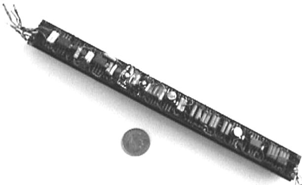
Figure 2 – Complete electronics for a well-logging probe used for pressure measurement in bore holes. This electronics operates to  $275^{\circ}\text{C}$  and with reduced life to  $315^{\circ}\text{C}$ . Below the electronics is a quarter for size reference. (Courtesy of Linear Measurements Inc.) [3]
