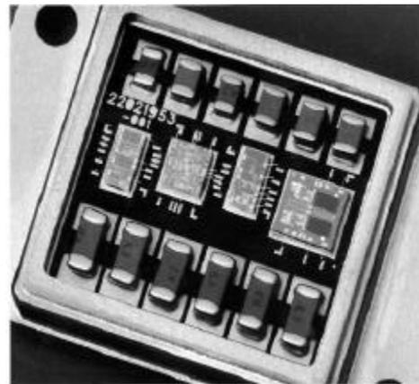
Figure 6 – A sensor interface circuit specified for several years operation at  $225^{\circ}\text{C}$ . It includes two silicon-on-insulator ICs, two resistor chips and 12 capacitors. (Courtesy of Honeywell Solid State Electronics Center.) [6]
