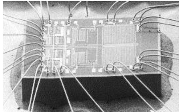
Figure 5 – A GaAs preamplifier IC for use in particle physics instrumentation. The die is  $2.5\text{ mm} \times 1.5\text{ mm}$ . This circuit can operate at temperatures down to within a few degrees of absolute zero. (Courtesy of the University of Milan.) [5]
