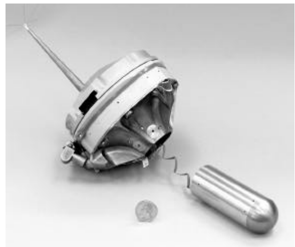
Figure 1 – A DS2 probe: the larger part (center) remains on the surface while the cylindrical part (lower right) penetrates up to about a meter into the Martian soil. Both parts contain low-temperature electronics. In the foreground is a quarter for size reference. (Courtesy of NASA/JPL/California Institute of Technology.)
