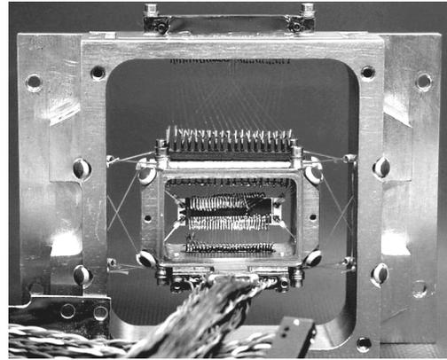
Figure 3 – A preamplifier assembly for X-ray detectors on the ASTRO-E satellite. The temperature of the outer frame is about 1.2 K ( $-272^{\circ}\text{C}$ ); of the innermost part carrying eight transistors about 120 K ( $-153^{\circ}\text{C}$ ). (Courtesy of NASA Goddard.) [4]
